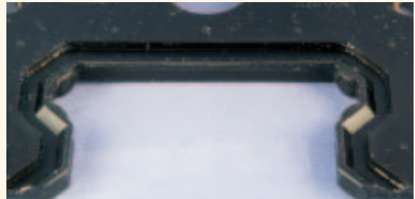
No.2 : LaCS installed on end seals: No abnormalities after traveling 5000 km
