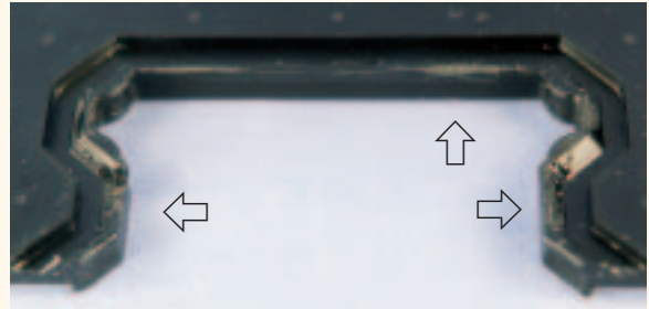
No.1 : End seals only: Damaged lip at 1700 km
