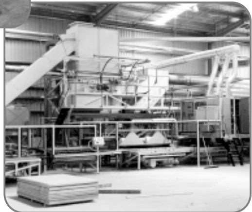
Pre-Feed and Stacking on Fibre Board Machine
