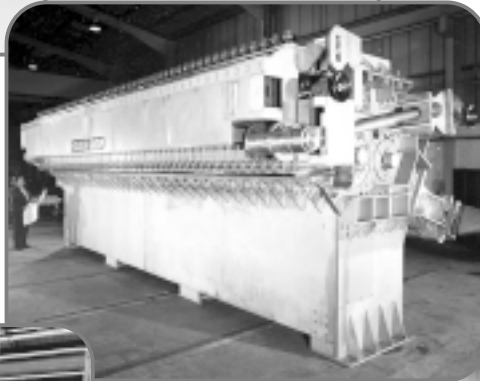
Headbox Adjustment on Paper Machine
